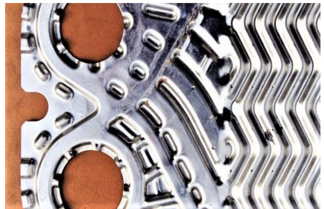
Fig. 8. AISI 316 steel HE plate pitting corrosion damage. Leaks were noted at the dark areas.
