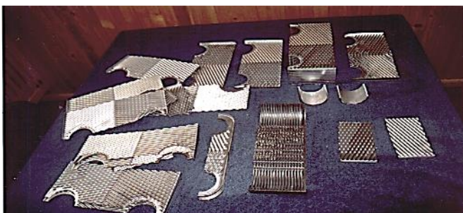
Fig. 10 Copper-brazed plate HE, cut and disassembled chemically in nitric acid
