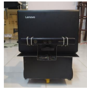
Fig. 8. Robot model with the Kinect RGB-D and PC.
